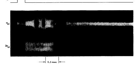
FIG. 8. Electrostatic signals from the Oak Ridge DCX-1 mirror machine which indicate the formation of a single cluster from the linearly stable regime. The modulation of the signal intensities is attributed to rotation in phase space of a cluster.
