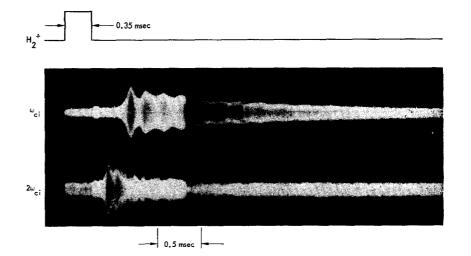
FIG. 9. Electrostatic signals from the Oak Ridge DCX-1 mirror machine which indicate the formation of two clusters from the linearly unstable regime. The second harmonic disappears and the first harmonic appears when two clusters coalesce into a single cluster.
